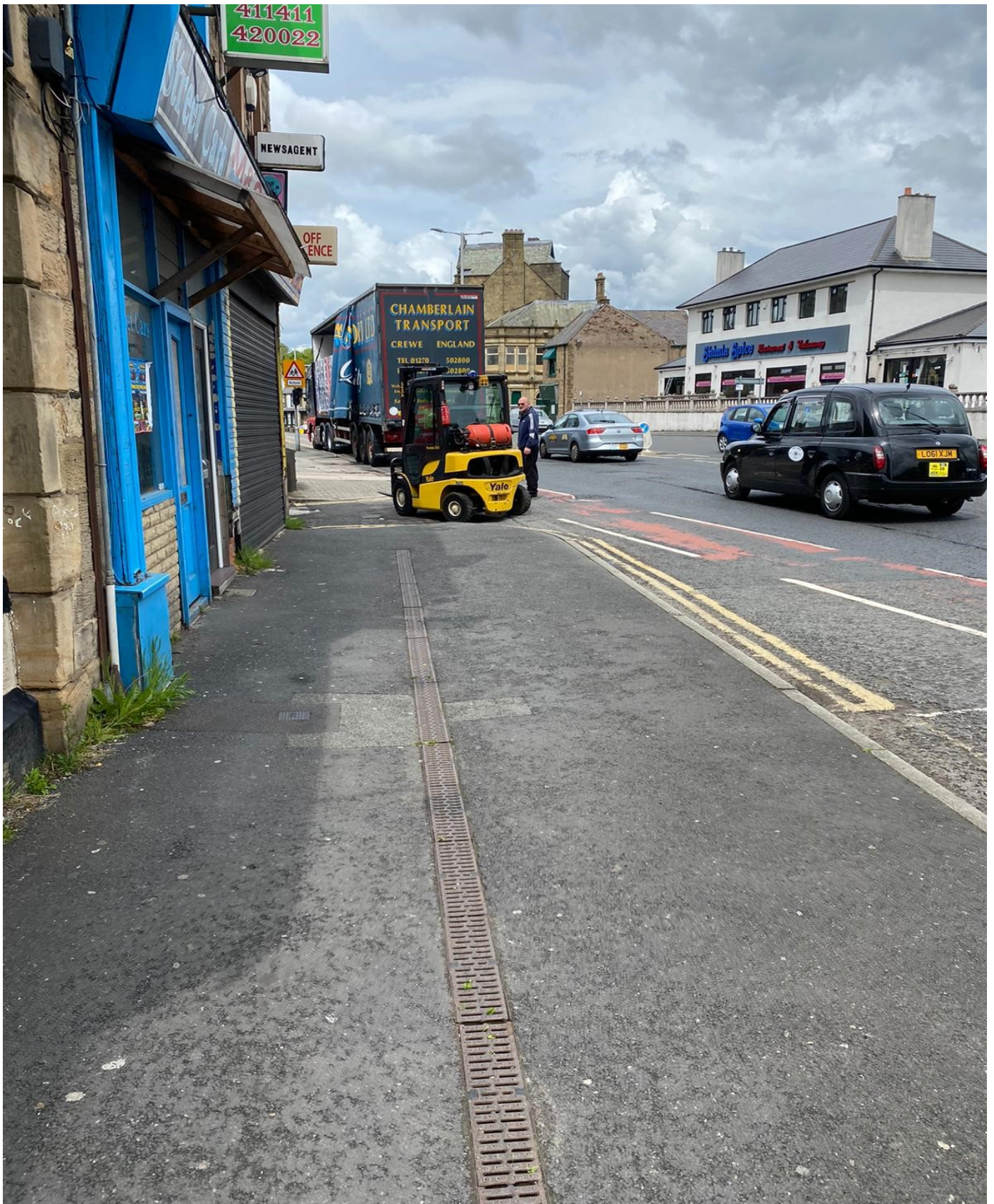
Using public footpath to operate Forklift on highway and causing obstruction for pedestrians. – Accident Hazard.
